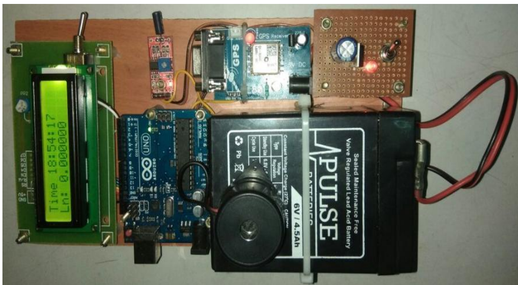
Figure 6. Hardware Setup of Speed Breaker detection System
